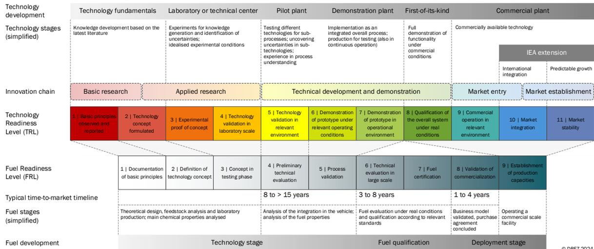
Figure 1 Overview of the Technology readiness level (TRL) and Fuel readiness level (FRL) (Hauschild et al. 2025)
