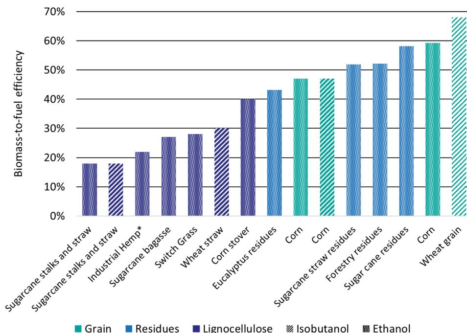
Figure 8 Biomass-to-Fuel-Efficiency of isobutanol to SAF and Ethanol to SAF value chains (\*SAF not final product), based on (Klein et al. 2018; Wang et al. 2021; Yao et al. 2017; Neuling and Kaltschmitt 2018; Tao et al. 2017; Cervi et al. 2021; Bullerdiel et al. 2019; Capaz 2021)
