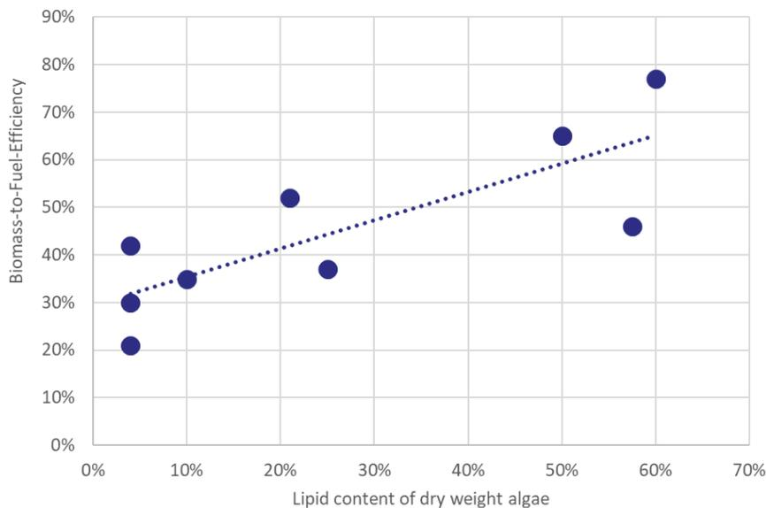
Figure 3 Biomass-to-Fuel-Efficiency of biocrude-oil to SAF pathways depending on the Lipid content of dry weight input-algae, based on (Farooq et al. 2020; Albrecht et al. 2016; Jones et al. 2014; Juneja and Murthy 2017; Barlow et al. 2016; DeRose et al. 2019)
