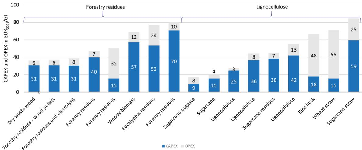
Figure 16 CAPEX and OPEX for different selected syngas to SAF value chains (Ahire et al. 2024; Cervi et al. 2021; Diederichs et al. 2016; Habermeyer et al. 2024; Jong et al. 2015; Kargbo et al. 2022; Michailos et al. 2017; Real Guimarães et al. 2023; Santiago et al. 2024; Wang et al. 2022)
