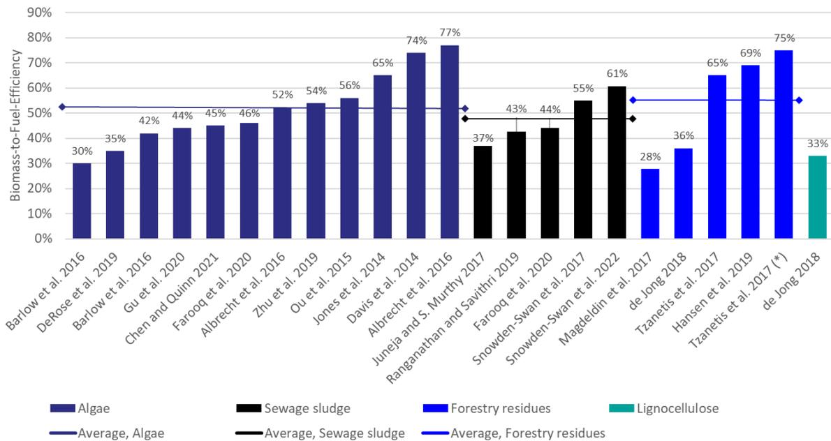
Figure 2 Biomass-to-Fuel-Efficiency of biocrude-oil to SAF pathways using different (\*SAF not final product within the study)
