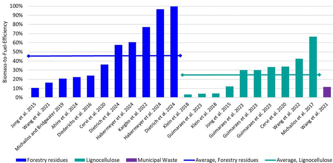
Figure 13 Biomass-to-Fuel-Efficiency of different selected syngas to SAF value chains
