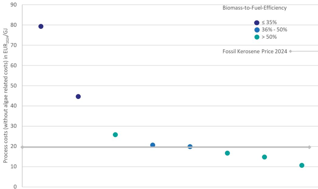
Figure 7 Process costs of biocrude-oil to SAF pathways from algae feedstock categorized by the Biomass-to-Fuel-Efficiency, based on (Barlow et al. 2016; Davis et al. 2014; Pedersen et al. 2018; Zhu et al. 2019; Gu et al. 2020; Jones et al. 2014; DeRose et al. 2019; EIA 2024)
