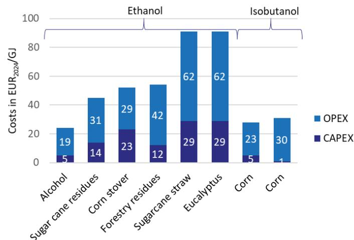
Figure 11 CAPEX and OPEX and specific production costs of isobutanol and ethanol to jet value chain, (Brandt et al. 2020; Capaz 2021; Cervi et al. 2021; Geleynse et al. 2018; Tao et al. 2017)
