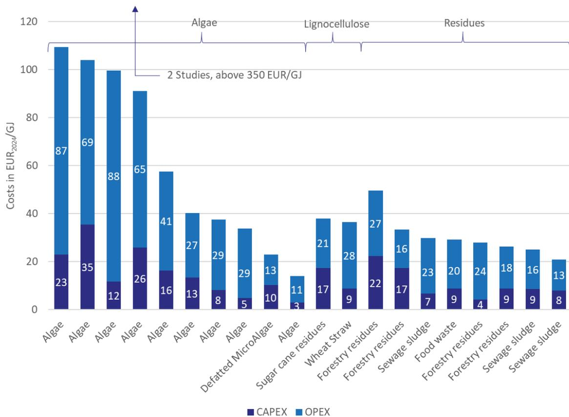
Figure 6 CAPEX and OPEX of biocrude-oils to SAF, based on (Albrecht et al. 2016; Barlow et al. 2016; Capaz 2021; Chen and Quinn 2021; Jong 2018; Farooq et al. 2020; Gu et al. 2020; Jones et al. 2014; Lippky 2017; Magdeldin et al. 2017; Nie and Bi 2018; Ou et al. 2015; Snowden-Swan et al. 2017; Snowden-Swan et al. 2022; Zhu et al. 2019)
