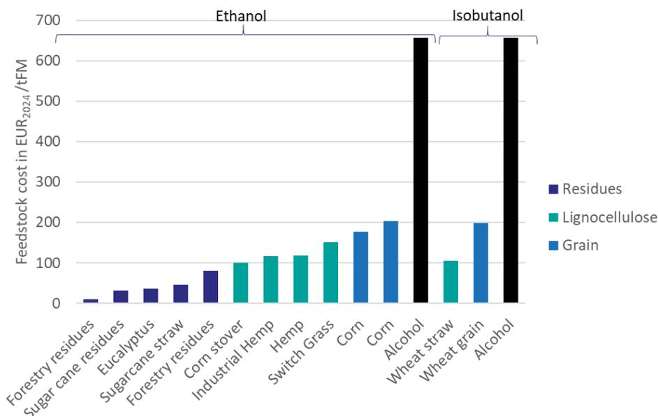
Figure 12 Feedstock costs sorted by feedstock categories, (Brandt et al. 2020; Capaz 2021; Cervi et al. 2021; Geleynse et al. 2018; Neuling and Kaltschmitt 2018; Tao et al. 2017; Viswanathan et al. 2021; Wang et al. 2021; Yao et al. 2017)
